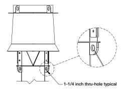
NOTE: Guy wires to be supplied by others. Fastening to building structure to be provided and engineered by others.
